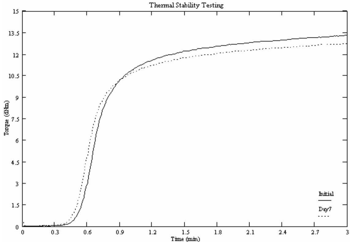
Figure 3: Rheometer Curves of material before and after 1 week at 71°C (160°F).
