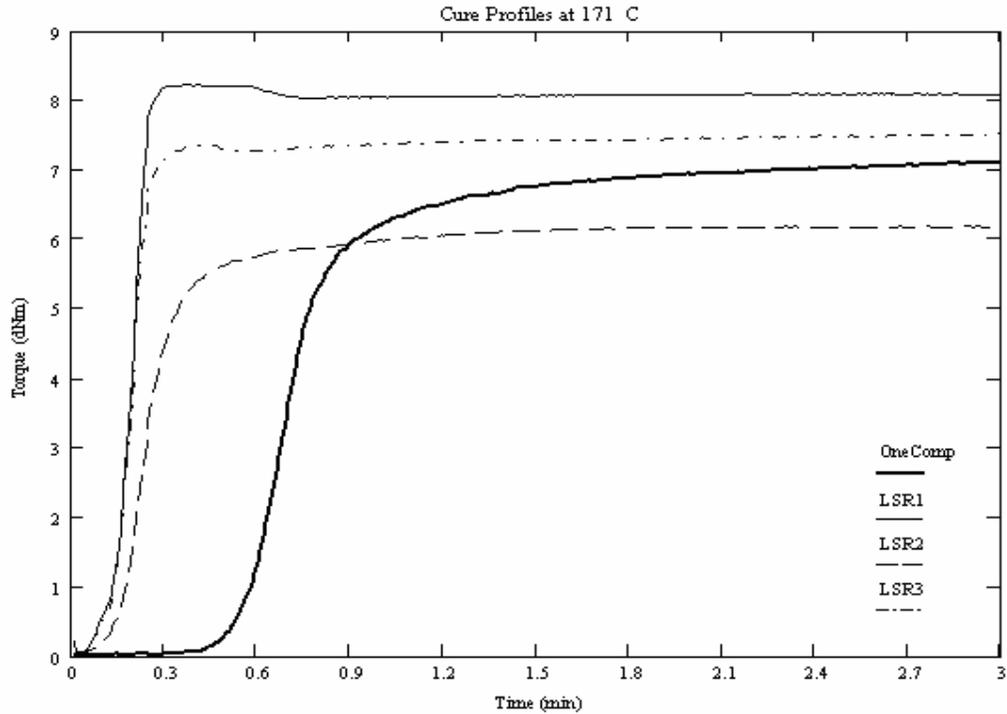
Figure 1: The Rheometer Curing of Liquid Silicones at 171°C (340°F)
