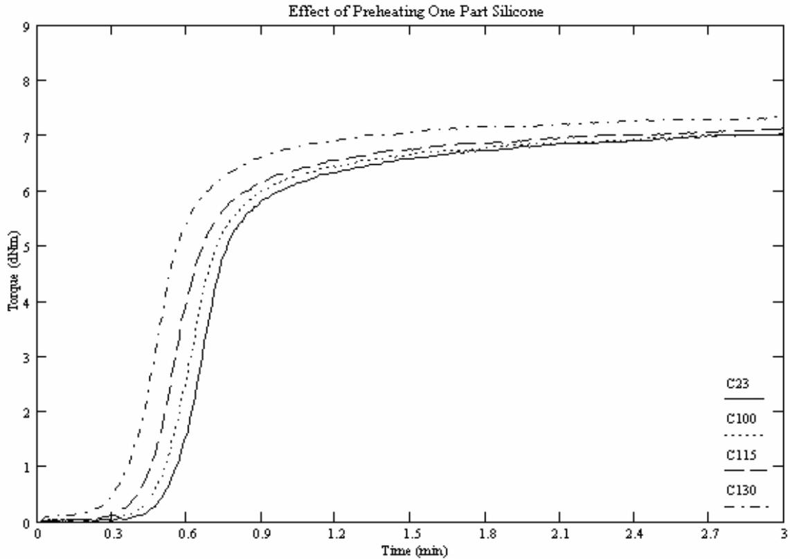
Figure 4: Rheometer Curves of ONE PART™ liquid silicone at various initial temperatures
