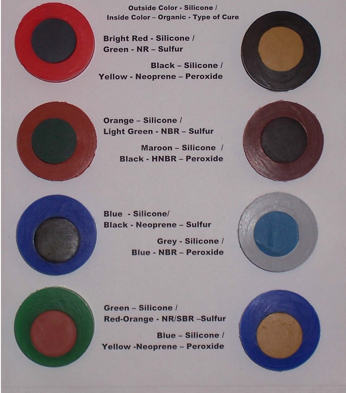
Fig. 3: One Part® LSR molded around cured organic rubber buttons
