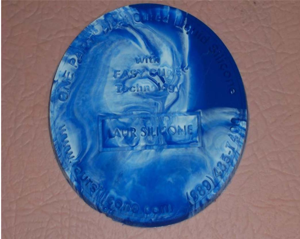
The equipment needed to do this will vary with the manufacturing method used. The coasters shown in the picture were made with a simple compression mold in a standard lab press.
