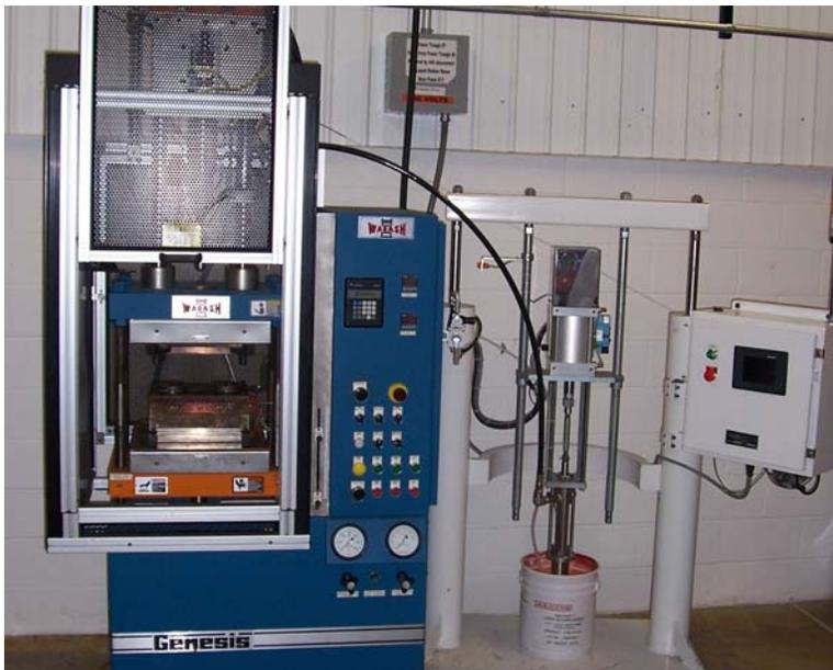
WABASH MPI Model GL30H-15-X Plunger Style Injection Machine is designed for use in a variety of LIM molding applications, including the use of ONE PART™ liquid silicone. Shown as run with two cavity semi-automatic mold.
